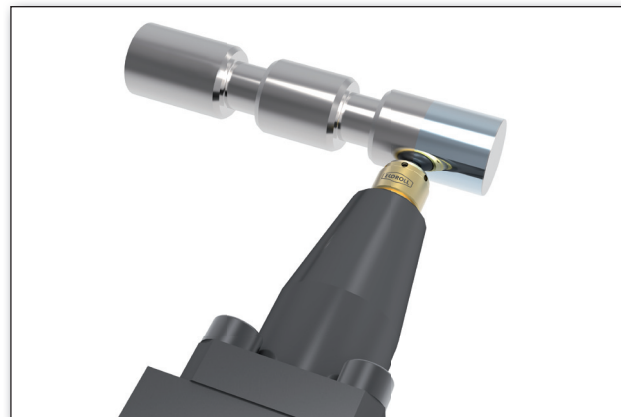
Deep rolling a control piston to increase its service life.
