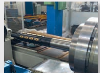
ZX-Tool on Deep hole drilling m.
