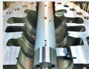
Recessing inside pump housing
