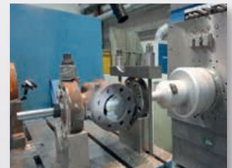
Machining seat pocket
